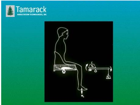
pressures than the ischia. Build a thigh fulcrum into the structural material of the seat cushion and put the footrest low enough so that the weight of the lower legs function like a lever to reduce pelvic contact pressures. This is impossible, of course, with an air flotation cushion.
