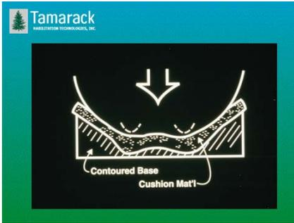
from bony, intolerant areas to areas of deeper soft tissue which is more force-tolerant. So, just like in a foot-bed or trans-tibial socket, a very good approach is to use a combination of shaping with only as much cushioning as is necessary because the user's position in the seat is not always perfect.
